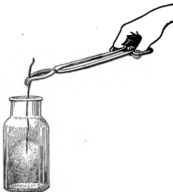
FIG. 84.— Burning Iron Wire in Oxygen.
